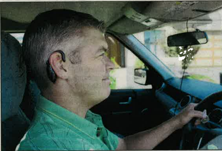
In action: When placed in the correct position the Driver Alert will activate once the driver's head falls forward, potentially preventing an accident.
