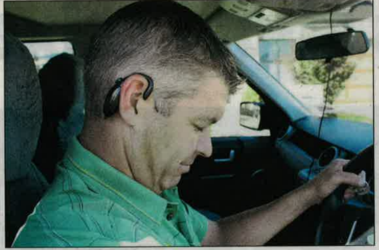
In action: When placed in the correct position the Driver Alert will activate once the driver's head falls forward, potentially preventing an accident.
