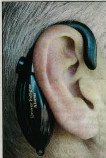
In place: The small device fits comfortably over the driver's ear.
